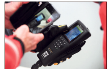
Lindsay Taylor uses a data sonde to analyze a water sample.
