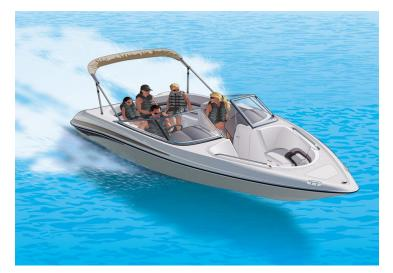
This is a planing hull because it looks like the boat is gliding over the surface of the water.
